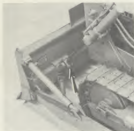
Lubricate 1 fitting on each lower trunnion. Total - 2 fittings.
