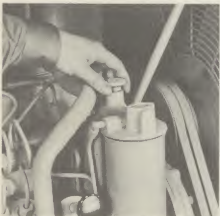
1. Move governor control to off position. Open vent valve.
