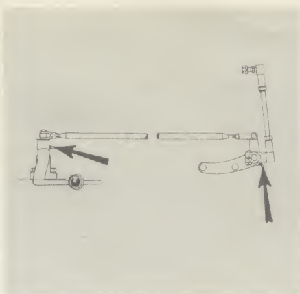
Lubricate 2 linkage pivots.
