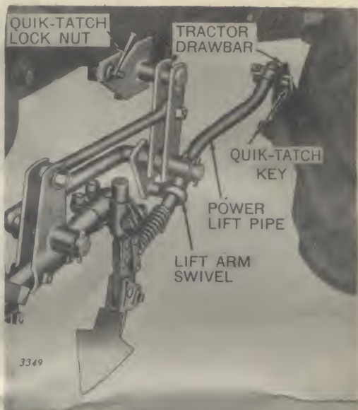
Figure 4—Attaching Front Rigs
