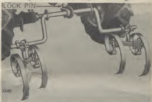
Figure 5—Attaching Rear Rigs
