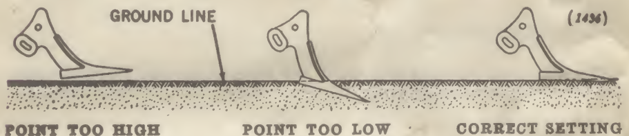
Figure 7—Setting Sweeps on Shanks
