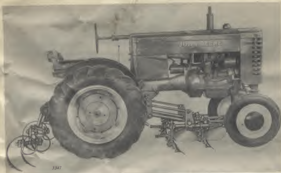
Figure 2—Cultivator in Working Position
