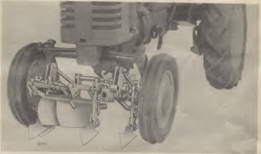
Figure 3—Driving Tractor Over Front Rigs
