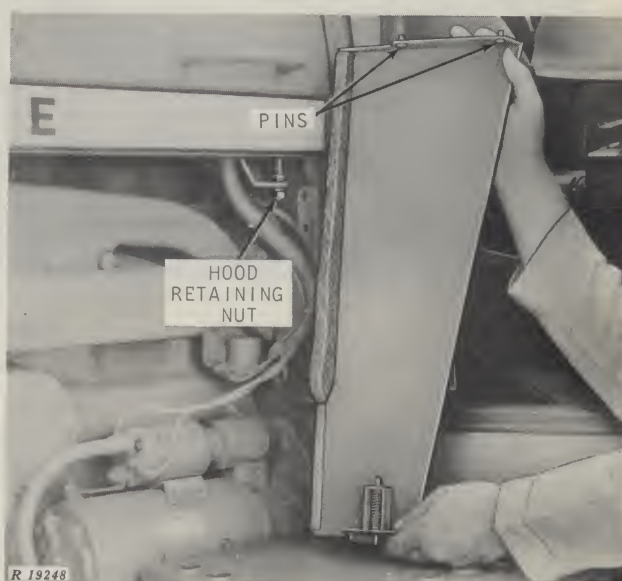
Removing Side Shield
