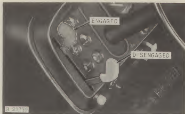
PTO Clutch Lever Operating Positions
