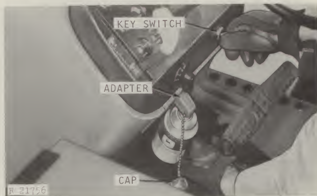
Injecting Starting Fluid
