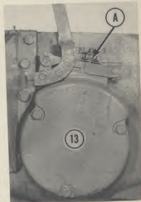
Fig. 0603A — Brakes on 4 speed and 6 speed tractors are adjusted by turning the nut (A). Item (13) is brake cover.
