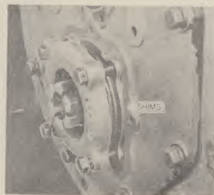
Fig. 0602—Removing bevel pinion shaft front bearing retainer from transmission front cover on Super 99 four speed tractor.
