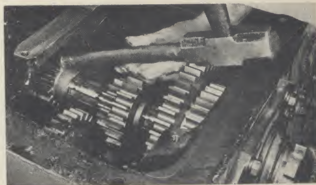
Fig. 0596—Bumping the spline (input) shaft of Super 99 four speed transmission backward prior to removal of shaft.
