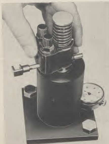
Fig. 0537B—Checking concentricity of injector spray tip to injector nut with GM tool J 5119.
