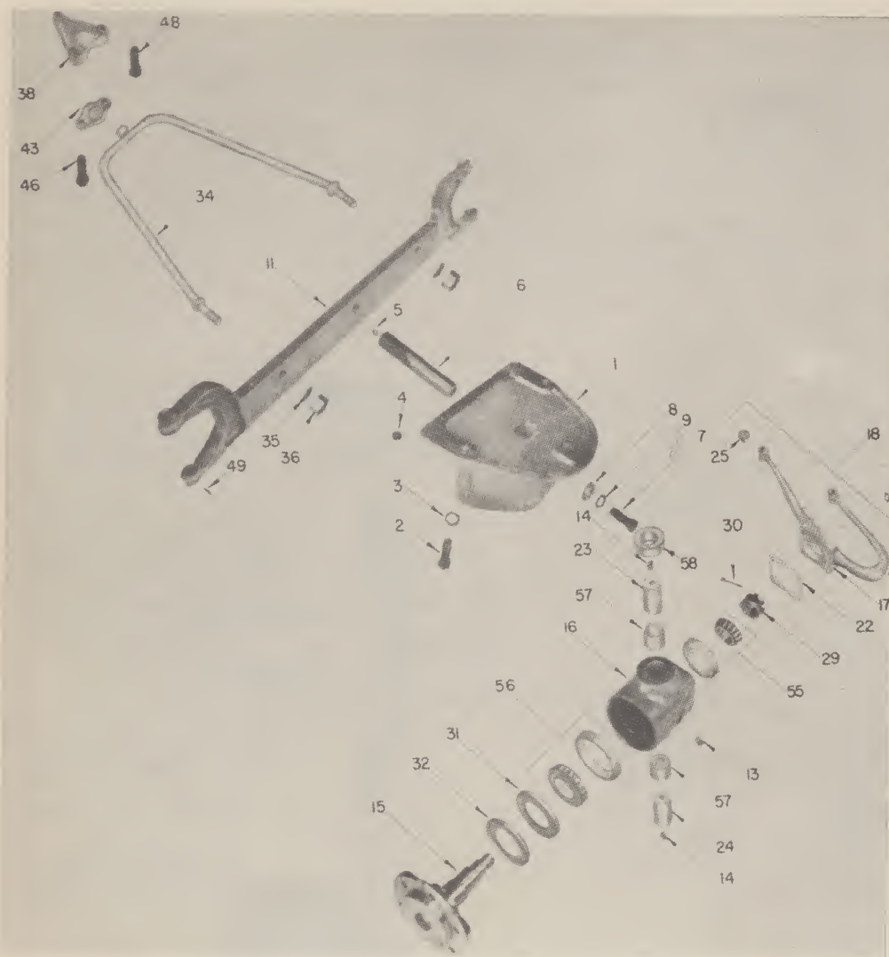
Fig. 0456A—Components of front axle, bolster, stay rod and one wheel spindle assembly. Spindle (15) is "live" type and rotates in spindle carrier (16).
