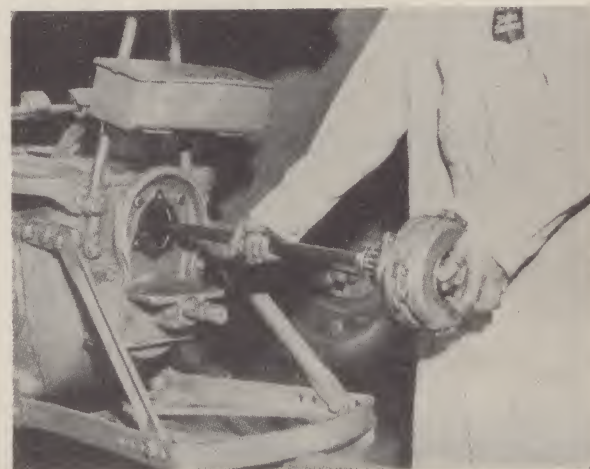
Fig. 0618 — Removing pto clutch and drive shaft assembly as a single unit.
