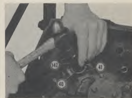
Fig. 0508A—GM engine. Showing method of installing an injector hole copper tube (40) with driver (142).
