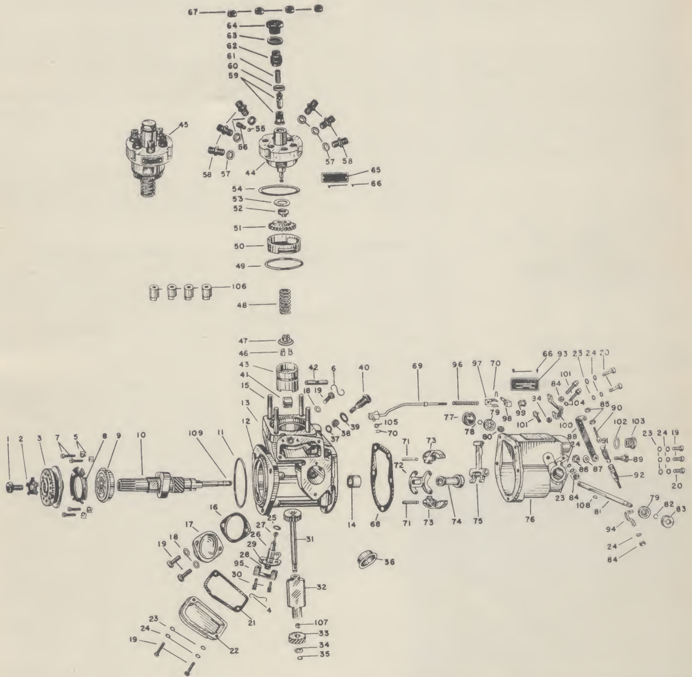
Fig. 0486—Disassembled view of Bosch PSB pump 6A70Y3826-A used on Super series tractors. Note round cornered hydraulic head assembly (45). Refer also to Fig. 0477.
